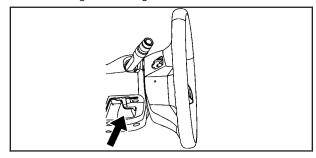
The tilt and telescope lever is located on the left side of the steering column.
